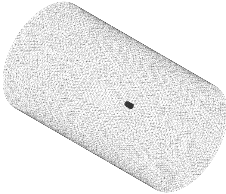
Figure 9. Mesh of the fluid volume used in the CFD analysis. The point in the center is where the EAPS is. It features a more dense mesh in that area due to the complex geometry.
